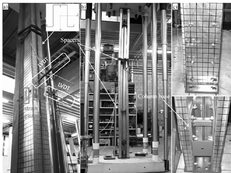
Figure 1 Experiments: (a) Column tests-specimens and equipment; (b) Columns-test setup and failure mechanism; (c) End connection
