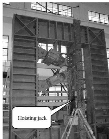
Figure 4 Test loading of KK-type joints
