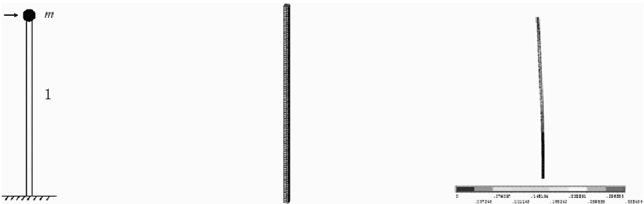
(a) Calculation diagram (b) FEA model (c) First-order mode
