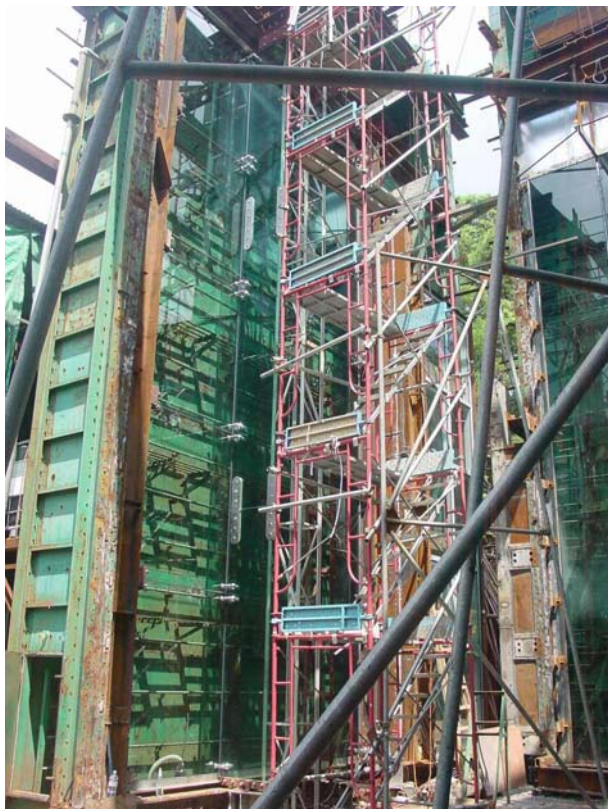
Figure 4: Glass Wall Specimen The glass is used as structural elements as glass fin.
