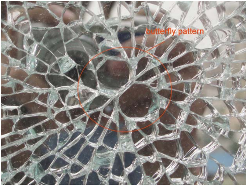
Figure 12: Spontaneous breakage of tempered glass
