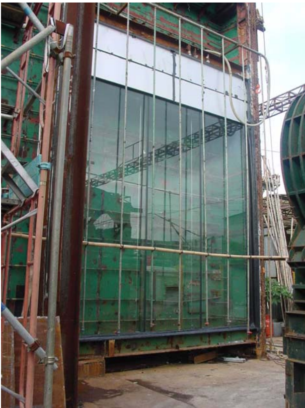
Figure 2: Glass Wall Specimen
