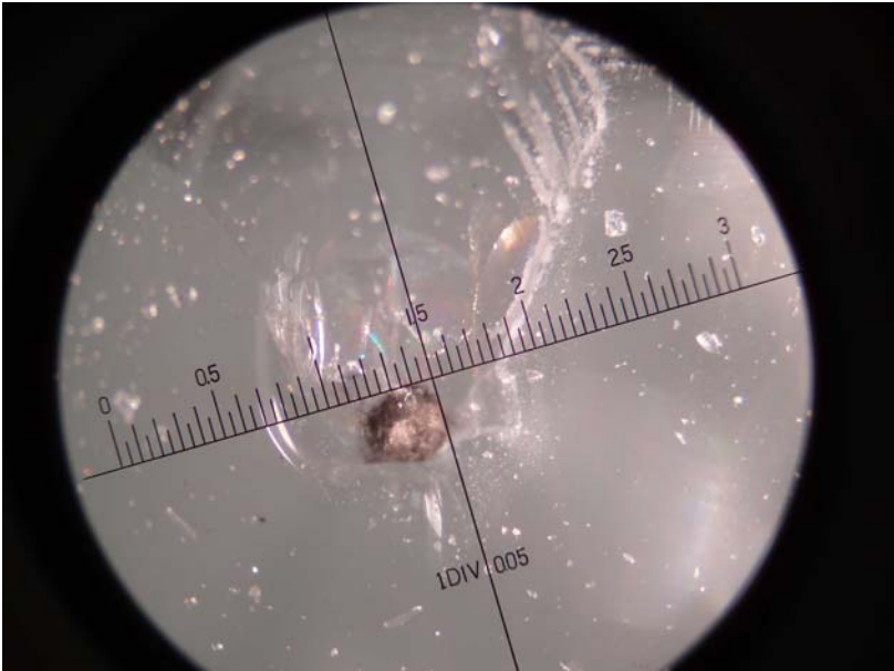
Figure 13: The inclusion (approx 0.35 mm dia.) found in the breakage origin (butterfly pattern)
