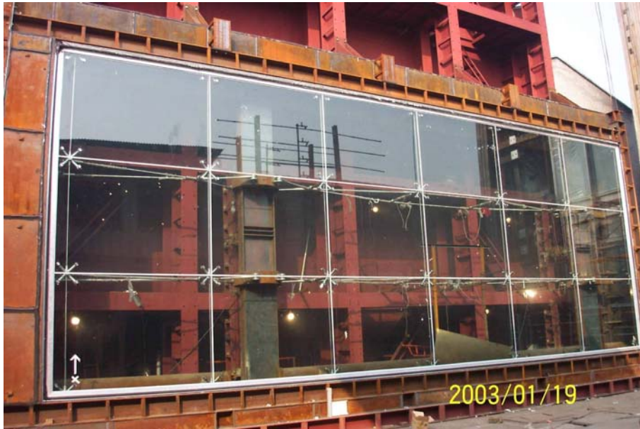
Figure 3: Glass Wall Specimen The facial glass is mechanically fixed to the tension rods.
