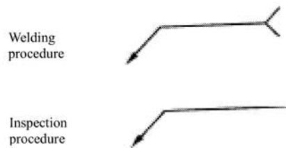
Figure 15 Conventional welding symbols giving welding and inspection procedure
